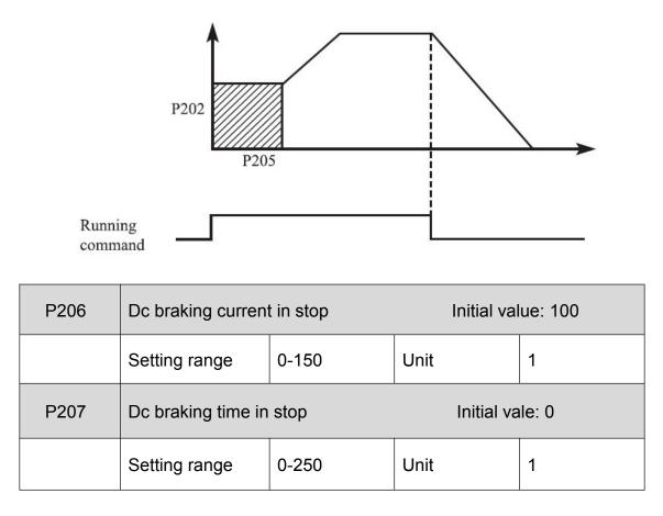
Dc braking in stop is application for load which has requirement on braking.
