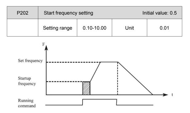
Start frequency is the initial frequency when inverter starts. For device with heavy load or requires large starting torque, increasing start frequency can make start easier. However, if the start frequency is too high, it may cause over current protection.
