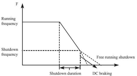
With regard to stop mode after stop frequency is reached, you can choose DC injection brake and other options. If you do not choose DC injection braking, it will stop in coasting stop mode.
