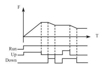
Explanation: when UP is valid (UP is closed), frequency will go up. When DOWN is valid (DOWN isclosed), frequency will go down.
