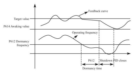
Example:PID action set point is 60% (0-100% is corresponding to 0-10V),and the wake-up value is 80%,which is actually corresponding to 0-10V,then the actual wake-up value is 60%×80%=48%(corresponding to 0-10V).
