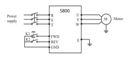
Parameter: P102=1 P315=6 P316=7 Operation Instruction of S800 series Inverter Actuation explanation:
