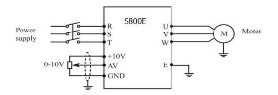
Explanation :control output frequency of inverter by AV voltage signal sent by external POT (10k  $\Omega$ )
