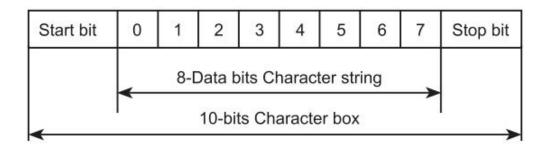
10-Bit character box (FOR RTU) Data pattern:8N1 for RTU
