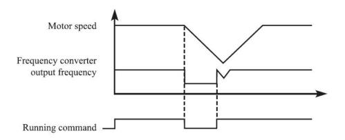
Attention: when inverter starts in tracing start mode, inverter will have speed tracing in the sequence of high to low frequency.
