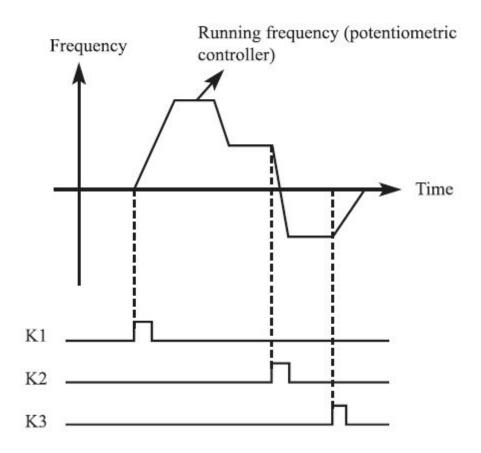
K1 forward rotation K2 reverse rotation K3 stop Output frequency is controlled by potentiometer.
