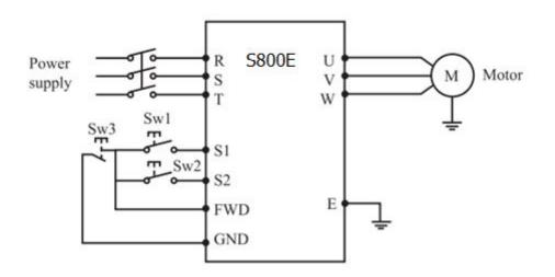
Use S1, S2,or S3 as input terminal for external signal Parameter: P317=6 S1 is in forward
