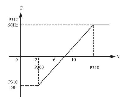
Introduction: P300=2 AV minimum voltage input: 2V (inverter regards signals below 2V as invalid signals);
