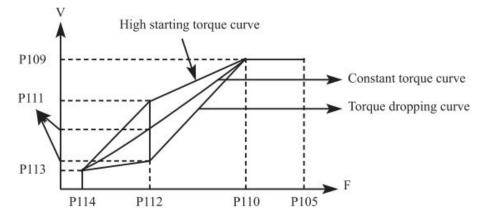
P109: V/F maximum voltage, V/F maximum voltage can be set .according to the motor connected. Generally, it will be set at the rated voltage of the motor .When motor is very near to inverter, usually within 30m, it should be set at a higher value.
