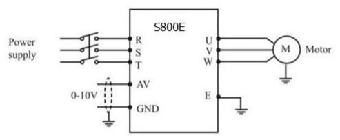
Explanation: control the output frequency through terminal AV/FC (0~10V)
