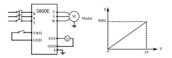
Parameter: P105=80.00 Max. frequency P106=0.00 Min. output frequency P306=0.00 FOV minimum voltage output P307=5.00 FOV maximum voltage output
