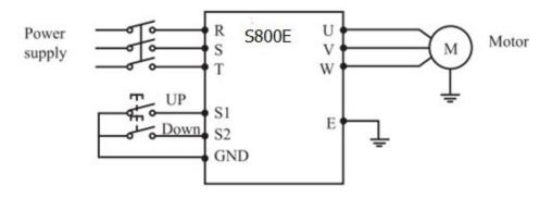
Parameter: P317=15, S1 terminal will be set in UP mode. P318=16, S2 terminal will be set in DOWN mode.
