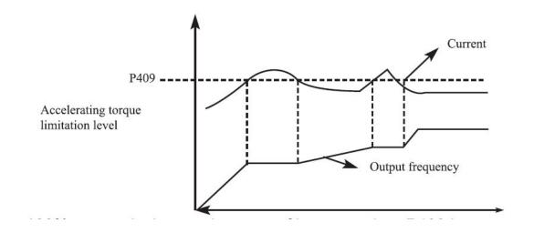
100% current is the rated current of inverter, when P409 is set to be 1, then accelerating torque limit is invalid, and it does not have protecting function.
